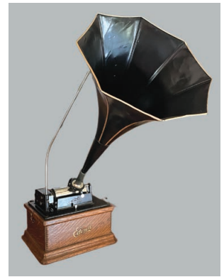
Above: This Edison "Fireside" phonograph could play both two- and four-minute wax cylinders.
