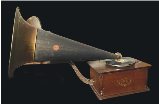
Above: A Kalamazoo Duplex phonograph. Available by mail order, this rare machine operated with a single reproducer using two horns.
